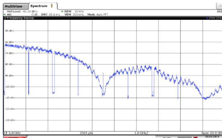
Figure 6 Broadband NPR with NRZ coding (notch at 4.5 GHz)
