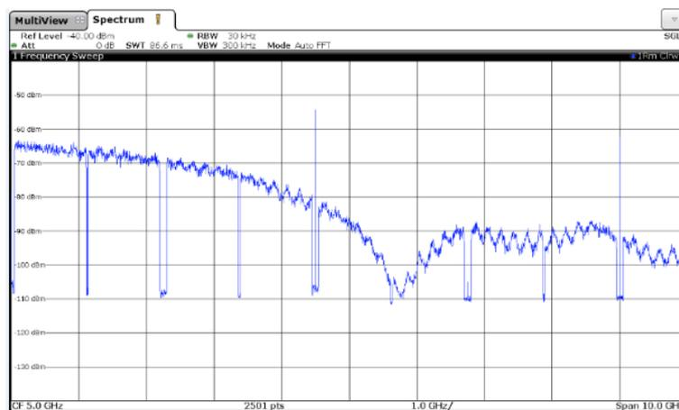
Figure 7 NPR with NRTZ coding (notch shifted to 5.7 GHz).
