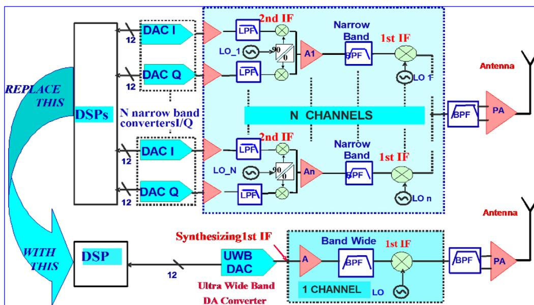
Figure 10 Contrasting a multi-carrier transmit path using baseband DACs (top), with using a single UWB DAC (below).
