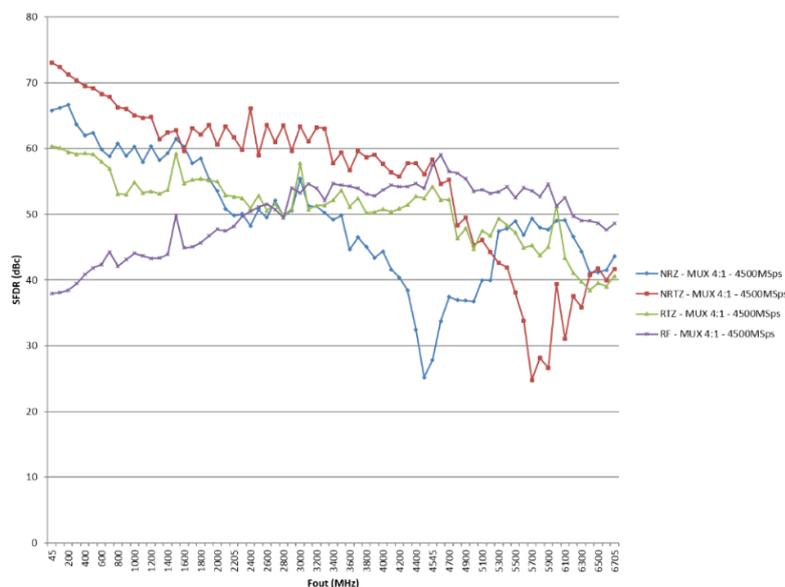
Figure 5 SFDR for each output mode of the EV12DS400.
