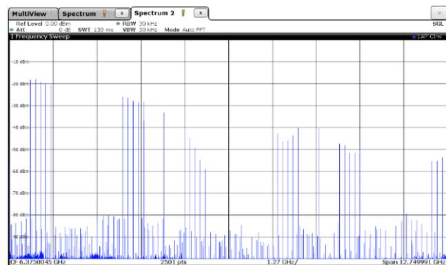
Figure 9 Multi-tone plot with signal maxima out to 12 GHz.
