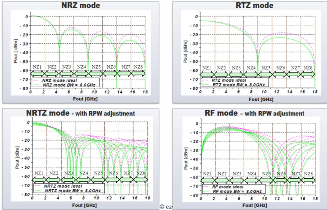
Figure 2 Frequency domain response plots of the four DAC output modes.
