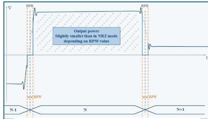
Figure 4 Sub-optimal RPW pulse width causes distortion.
