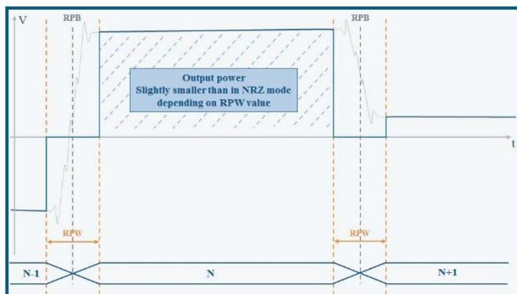
Figure 3 RPW showing optimum pulse duration.
