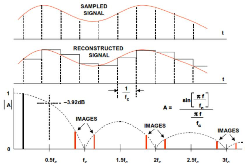
Figure 1 Waveform sampling in the time and frequency domain. Lower plot show alias signals extending out to > 13 GHz.
