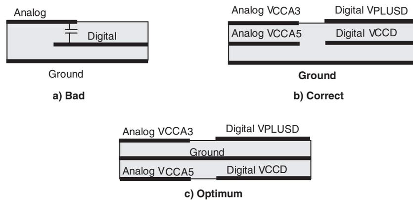
Since DGND and AGND are separated on package and chip, a continuous low impedance ground plane can be used for both Digital and Analog ground.
