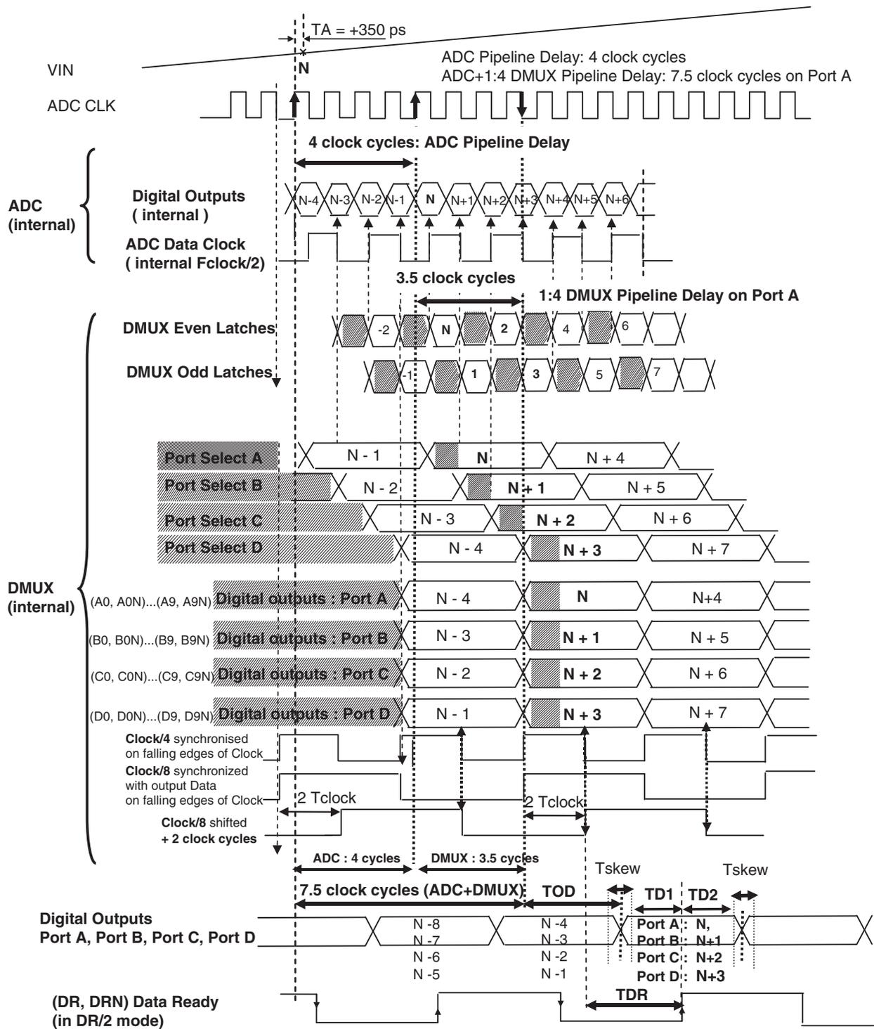
Figure 2-21. Timing Diagram Staggered Mode, 1:4 DMUX Ratio
