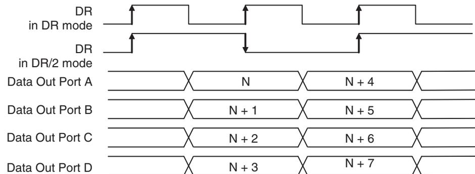
**Figure 4-9.** Simultaneous Mode in 1:2 Ratio (STAGG = 1)
