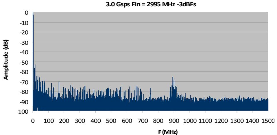
**Figure 2-18.** FFT 3.0 Gsps Fin = 2995 MHz @-7 dBFS (Carrier at end of the 2nd Nyquist Zone is folded back to baseband)
