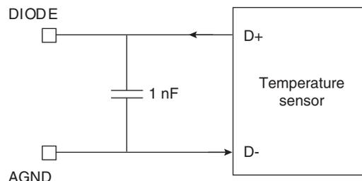
Diode pin is provided so that the diode can be probed using standard temperature sensors.
