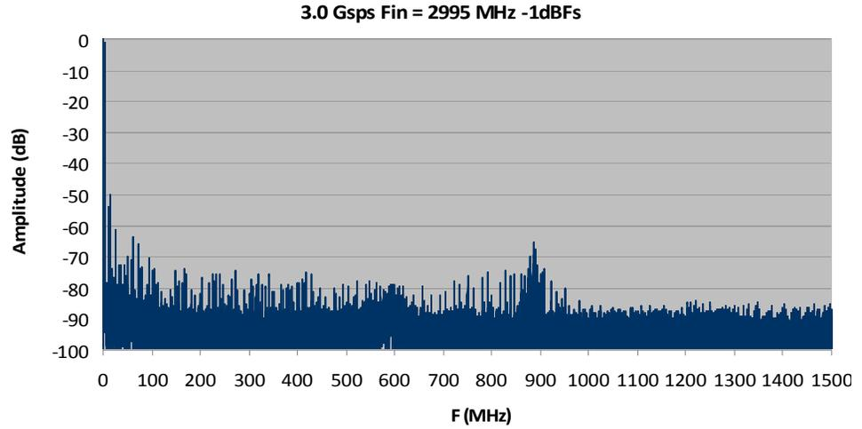
**Figure 2-17.** FFT 3.0 Gsps Fin = 2995 MHz @-3 dBFS (Carrier at end of the 2nd Nyquist Zone is folded back to baseband)
