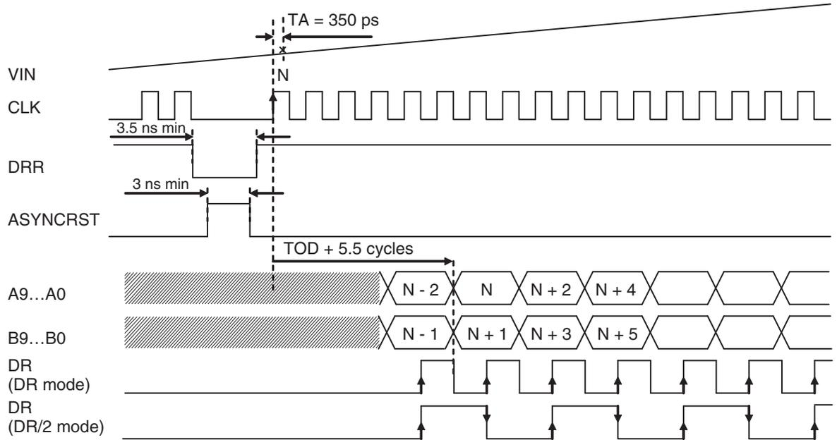
**Figure 4-2.** Asynchronous Reset Timing Diagram, 1:4 mode, simultaneous mode (Principle of operation)
