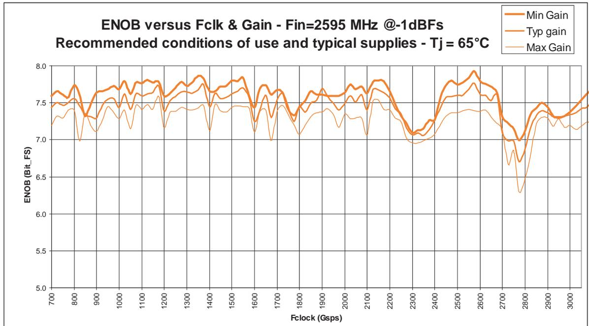
When a single tone sinewave at level of around -6 dBFs is applied, a SNR reduction may be observed by typically #6-8 dB resulting in ENOB decrease (#-0.8 bit). (No impact on THD/SFDR). In time domain the "glitches" that may be observed in this condition are 32 LSB maximum. Their potential occurrence is reduced with minimum gain and minimum VCCA5 and higher temperature. Low Fin (1st Nyquist) and/or low Fclk Frequencies are also more favourable cases.
