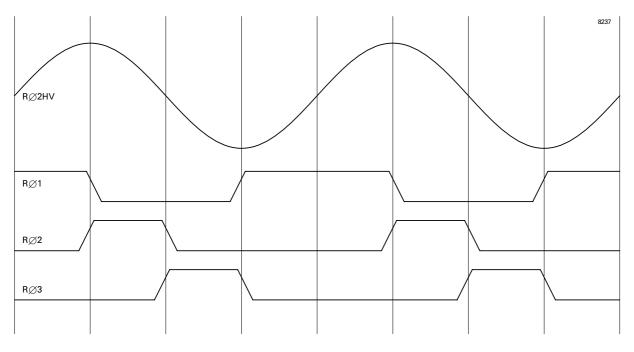
Figure 6: CLOCKING SCHEME FOR MULTIPLICATION GAIN (Conventional clocking scheme) (see note 16)
