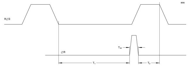
$T_W = 10 \text{ ns typical}$   $T_1 = \text{output valid}$  $T_2 > 0 \text{ ns}$
