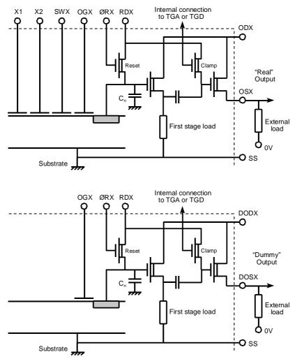
The first stage load of each output (real or dummy) draws a quiescent current of approximately 0.3 mA.
