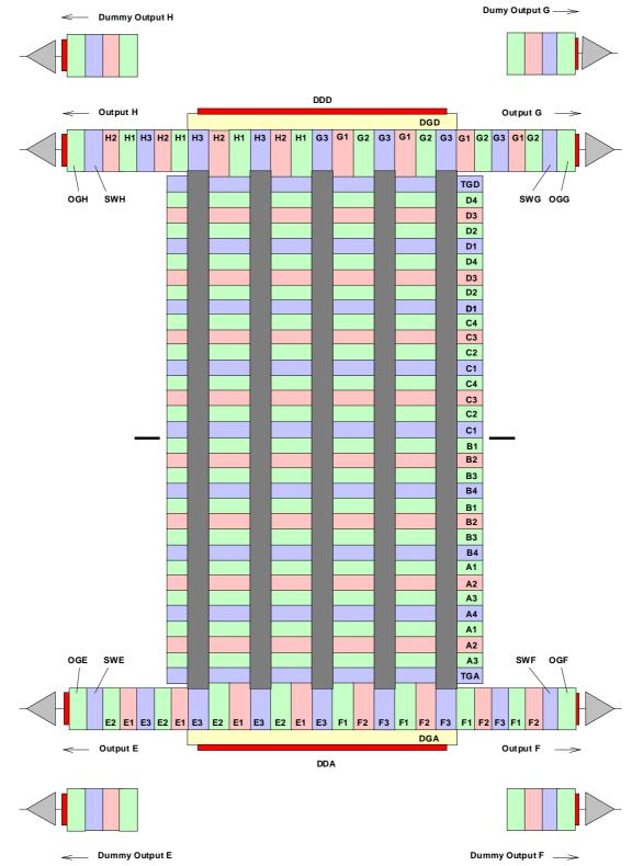
The IMO implant is under image phases A4, B4, C1, D1 and the transfer gates as shown below.
