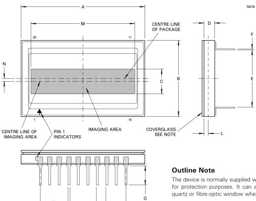
The device is normally supplied with a temporary glass window for protection purposes. It can also be supplied with a fixed, quartz or fibre-optic window where required.
