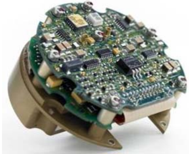
ESAU Electronics Assembly with removable EFI detonator for missile application
